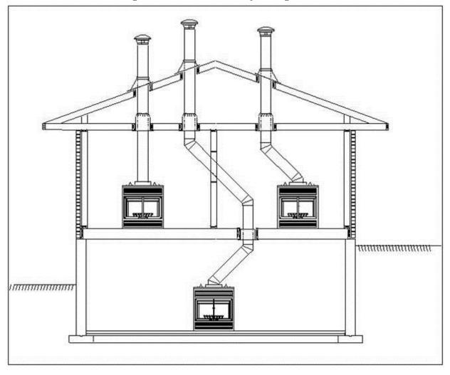
Figure #2: Possible Chimney Configurations
