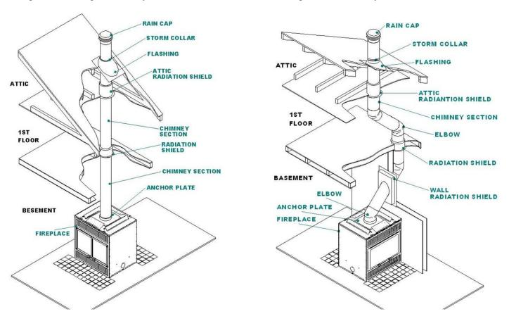
Figure #9: Exterior chimney installation
