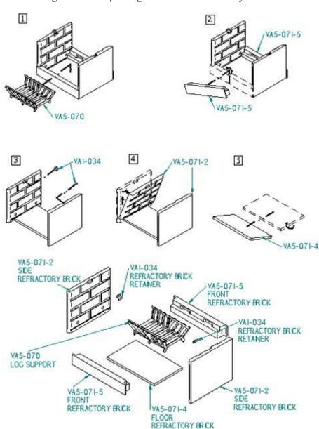
Figure #15: Replacing Westmount refractory bricks
