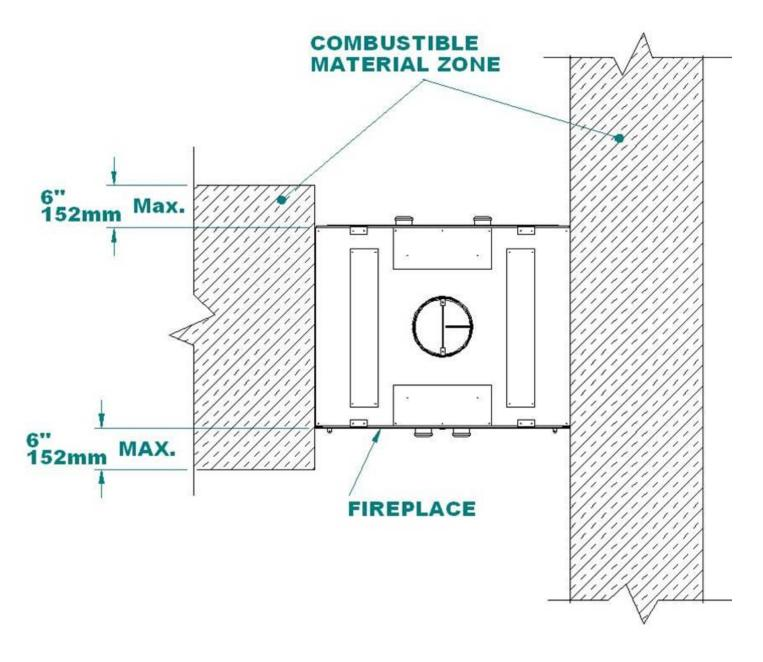
Figure #12: Chimney Enclosure 84" 2134mm Min. **ENCLOSURE** FRONT VIEW MODEL 2 CHIMNEY ENCLOSURE 84" 2134mm Min. CHIMNEY ENCLOSURE SIDE VIEW 84" 2134mm Min. FRONT VIEW MODEL 1
